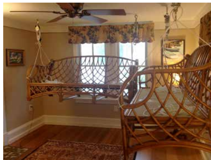
Figure 8: A pulley system lifts heavy or bulky furniture above predicted flood waters. All other contents can be moved to upper levels of the house. Photo: Mary Delaney Krugman, JD, MSHP
